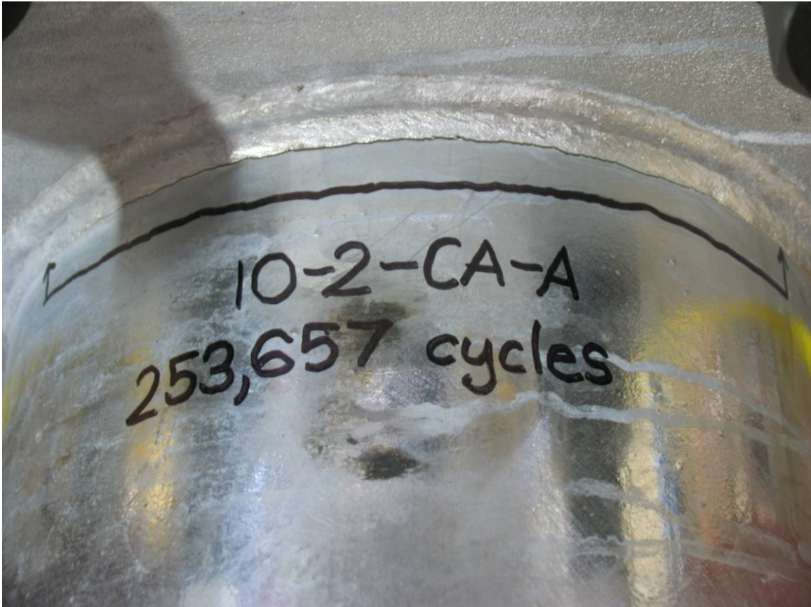
Figure 6.6 Typical Failure of the California Weld Profile Socketed Connection
