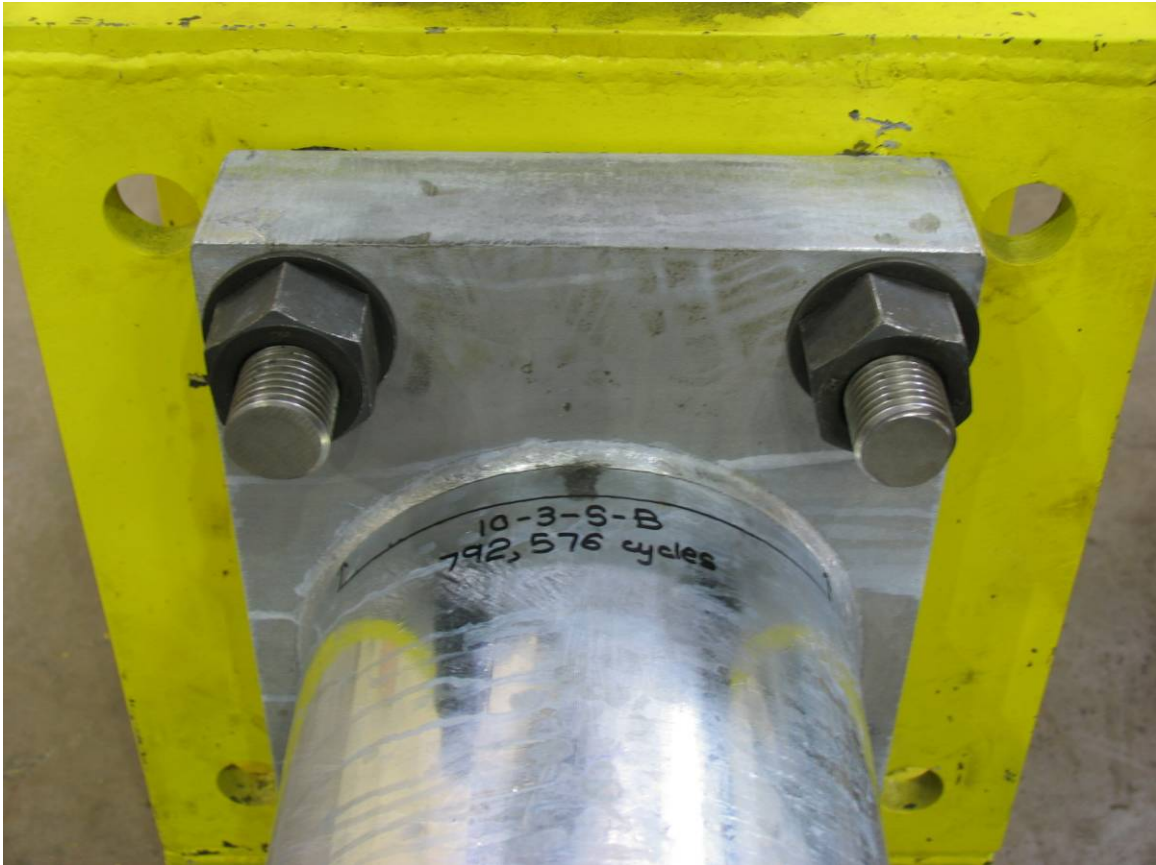
Figure 6.1 Typical Failure of the Standard Socketed Connection
