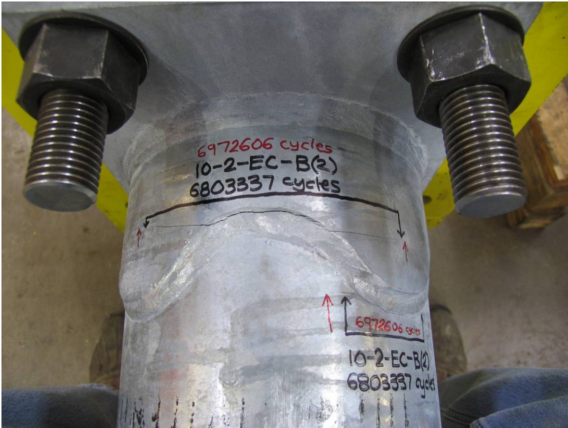
Figure 6.12 Exception to Typical Failure
