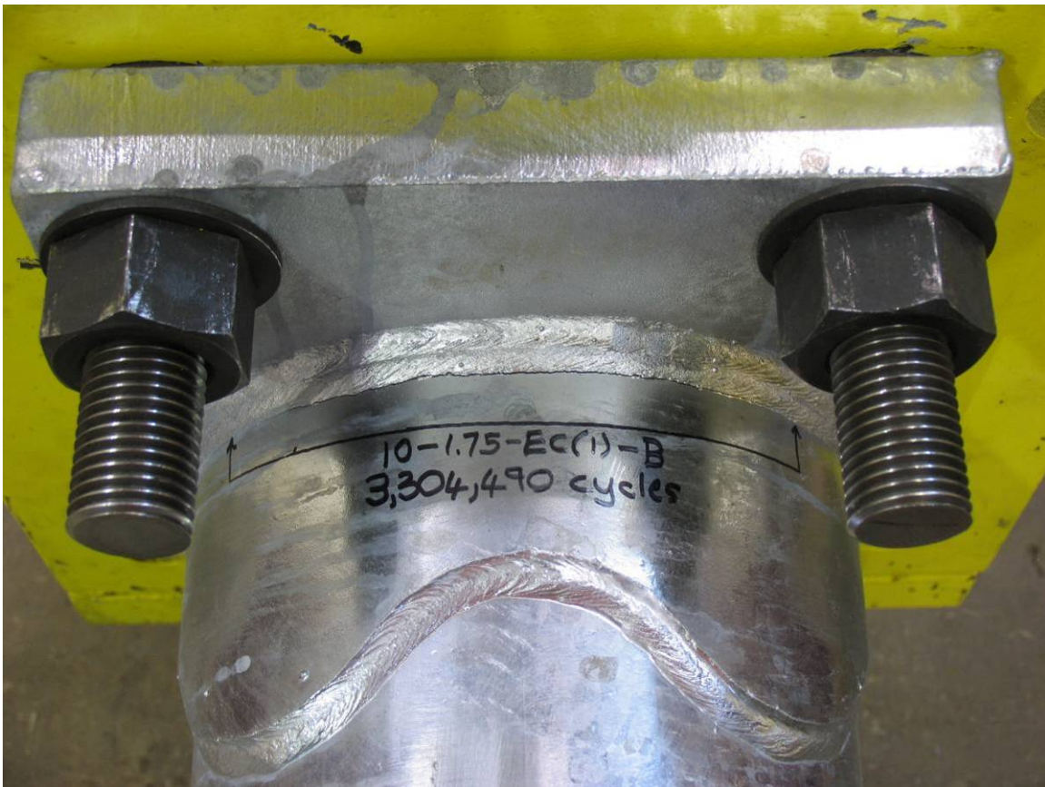
Figure 6.8 Typical Failure of the External Collar Specimens
