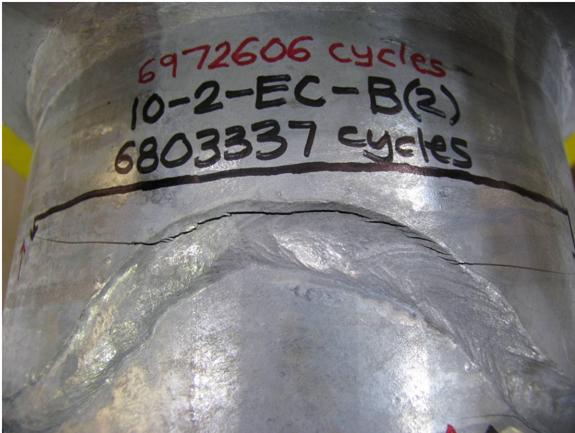
Figure 6.14 Fatigue Crack at External Collar Minimum Dimension
